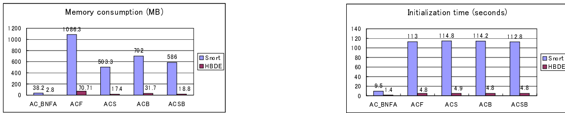
Fig. 3. Comparison of memory consumption (left) and initialization time (right) in different string pattern matching algorithms
